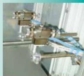
Mountings for PILOT WA 800: • Mounting flange to attach the adapter plate to the gun.
