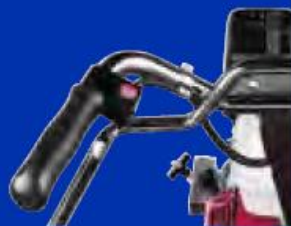
Electric Gun Control —Manual or automatic paint and bead guns with a push of a red button.
