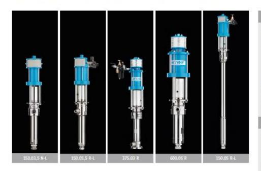
These new low pressure pumps still use the well proven WIWA compressed air motors. The transfer pumps differ from their predecessors by the following features: Revolving piston gland packing with four V-sleeves, easy assembly and disassembly, low weight, the piston is simply hooked in, as with the Airless paint spraying units.
